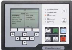
The PowerCommand control system is an integrated microprocessor based generator set control system providing voltage regulation, engine protection, alternator protection, operator interface and isochronous governing. Masterless Load Demand-capable generators are equipped with an additional s-CAN network connection that allows sharing of information amongst paralleled generator sets. MLD has been designed for hassle-free installation, commissioning and operation.
